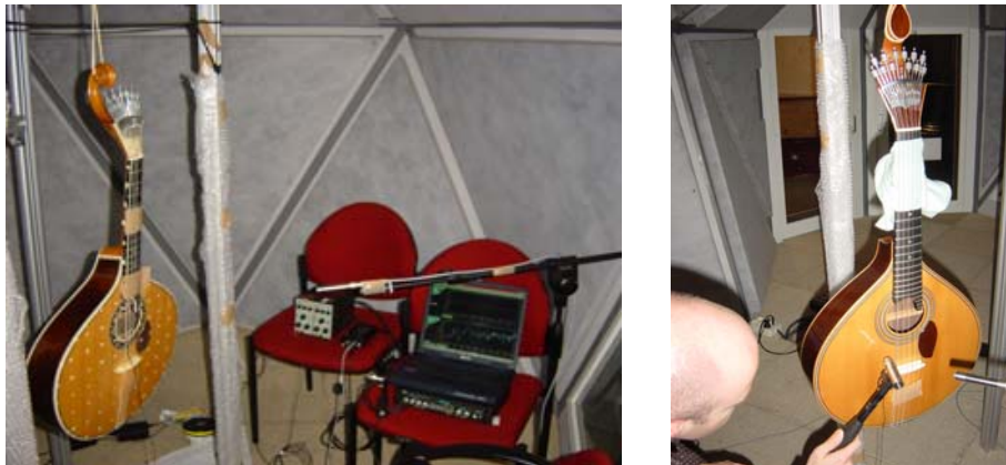
Figure 2 – Experimental setup showing the impact test positions and the location of the microphone for the vibroacoustic transfer functions measurements.
