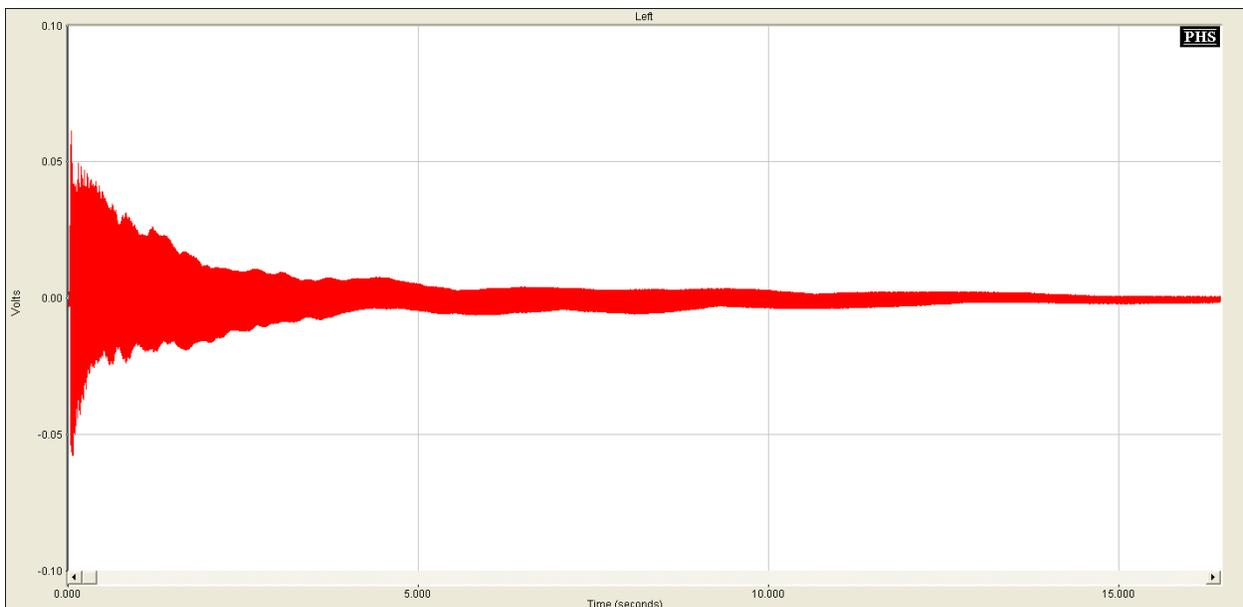
**Figure 1: Amplitude spectra (Volts vs. time) low E calibration file for Fender Texas Special pickup.**
