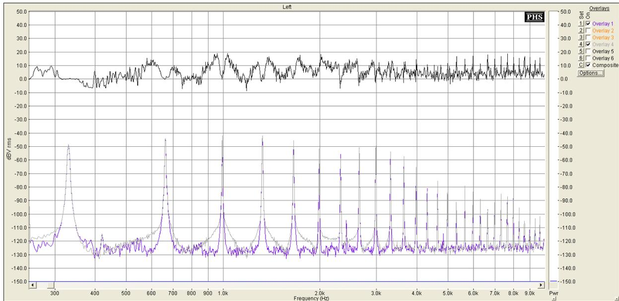
Figure 9: High e string frequency spectra (db vs. Hz) for Gibson 57 pickup. MMM in purple, AMM in gray, difference in black.
