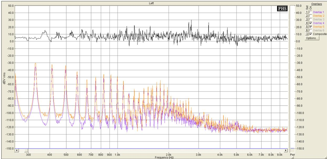
Figure 4: Low E string frequency spectra (dB vs. Hz) for Ash-MapleMaple guitar. Gibson 57 in purple, JB in orange.
