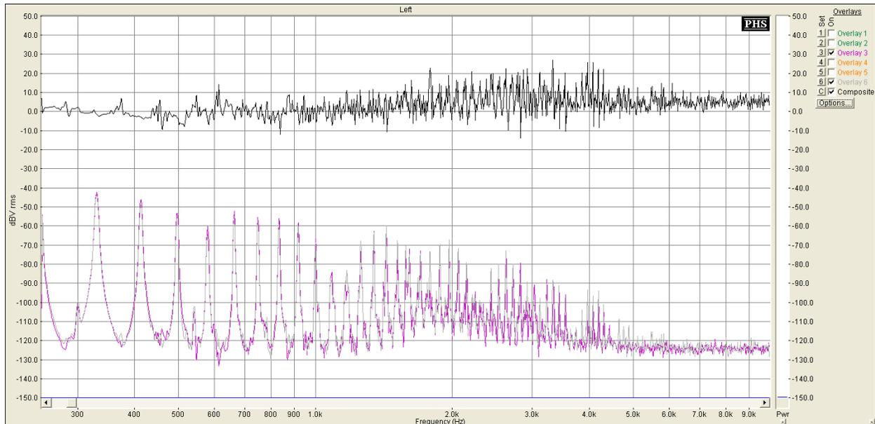
Figure 8: Low E string frequency spectra (dB vs. Hz) for Texas Special bridge pickup. MMM in purple, AMM in gray, difference in black.
