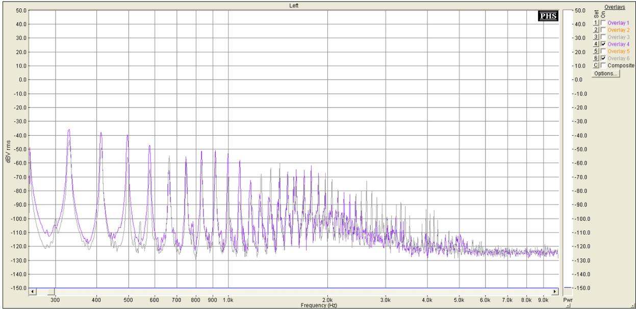
Figure 3: Low E string frequency spectra (dB vs. Hz) for Ash-MapleMaple guitar. Texas Special in gray, Gibson 57 in purple.
