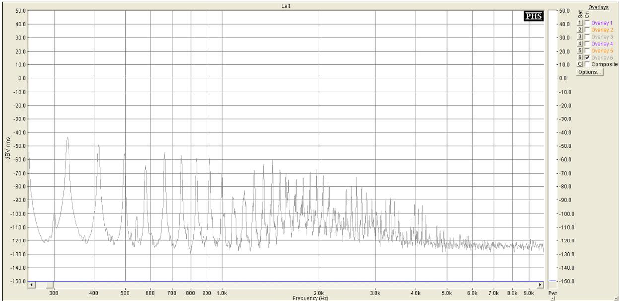
Figure 2: Low E string frequency spectra (dB vs. Hz) for Ash-MapleMaple guitar. Texas Special pickups in gray.
