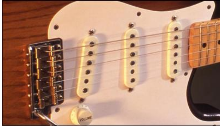
Figure 18. Bridge, middle and neck Stratocaster pickup locations.
