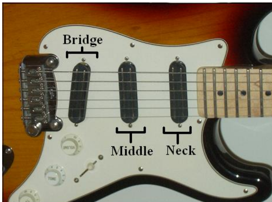
Figure 1. Pickup locations on a guitar affect tonal characteristics of pickup output.
