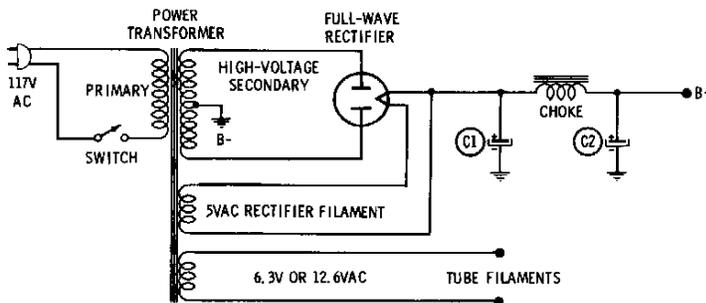
Fig. 3-6. Transformer power supply with full-wave rectifier.
