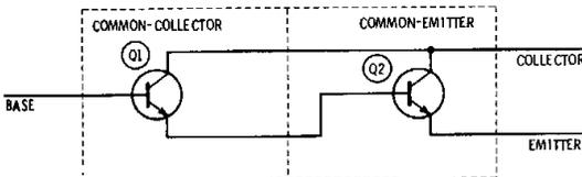
Fig. 1-14. Darlington pair—two transistors in one case.
