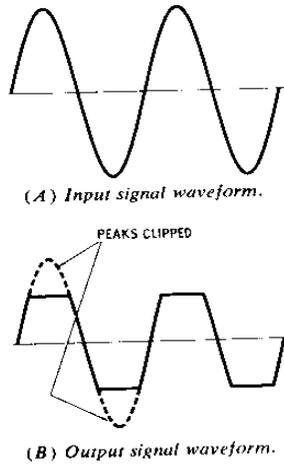
Fig. 2-21. Input and output signals of a "fuzz-box."
