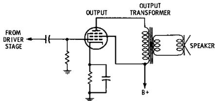
Fig. 1-5. Schematic of a single-ended power-output stage.
