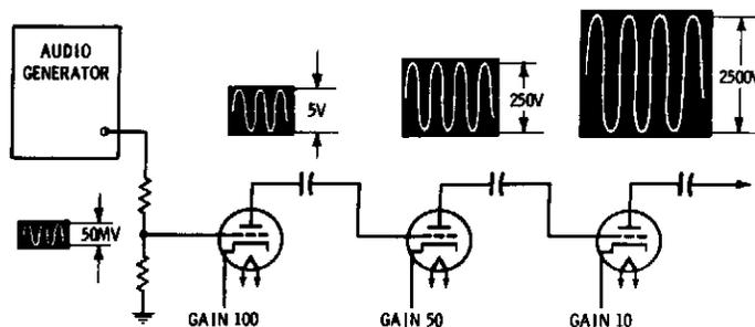
Fig. 8-5. Possible waveform values and stage gains.
