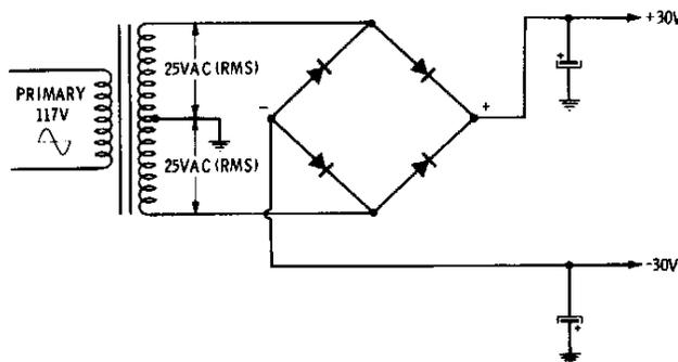
Fig. 3-9. Dual-polarity power supply.
