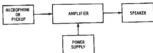
Fig. 1-3. Block diagram of a typical guitar assembly.
