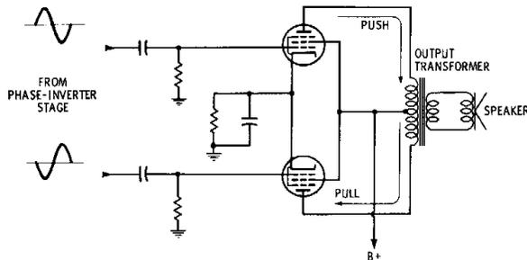
Fig. 1-6. Two-tube push-pull stage.
