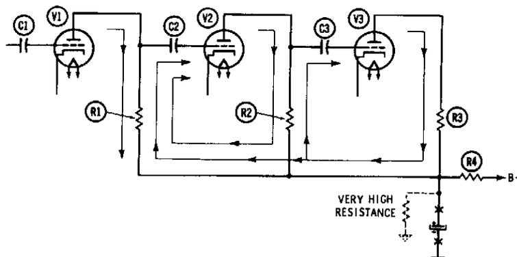
Fig. 8-7. Signal paths when bypass capacitor opens.
