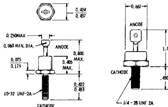
Fig. 5-10. Stud-mount rectifiers used in heavy duty amplifiers.
