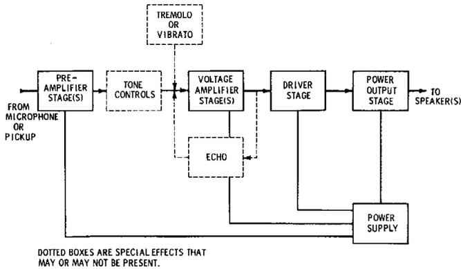
Fig. 1-4. Block diagram of a typical guitar amplifier.
