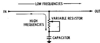
Fig. 2-5. High-cut tone-control circuit.
