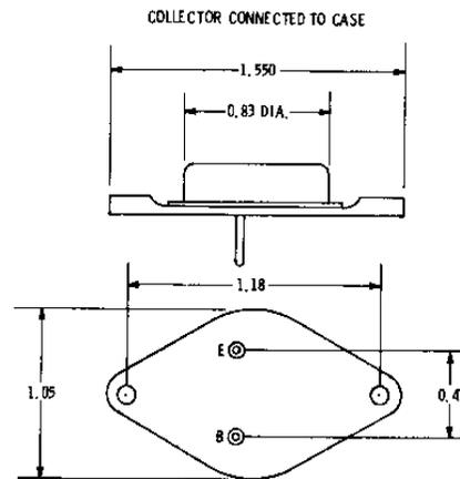
Fig. 4-9. The TO-3 case used for high-power transistors.
