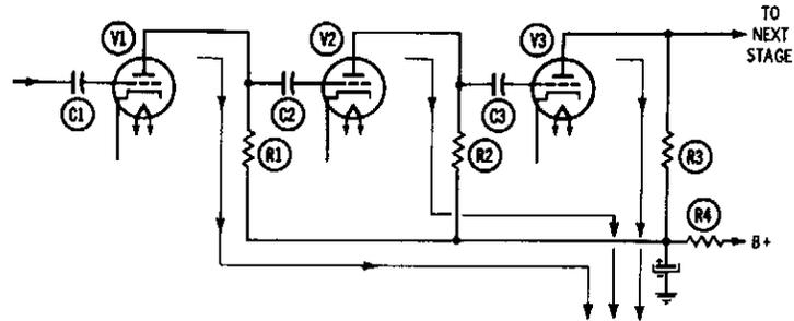
Fig. 8-6. Normal signal paths to ground.
