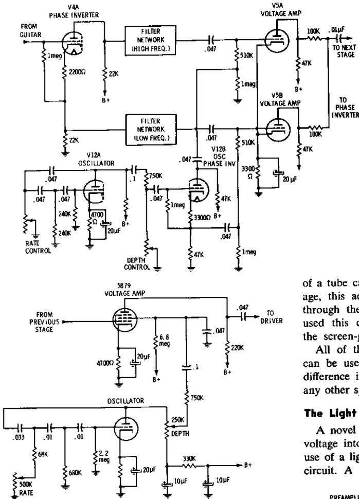
Fig. 2-9. Tremolo applied as two out-of-phase signals.
