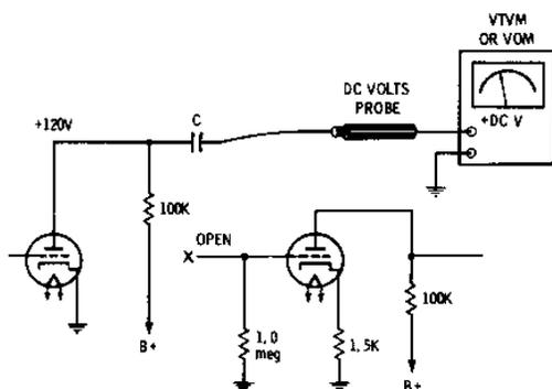
Fig. 4-4. Testing a coupling capacitor for leakage.
