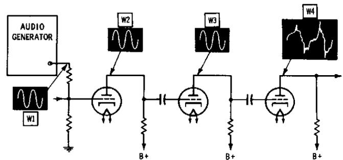
Fig. 8-2. Waveforms at critical points in an amplifier.
