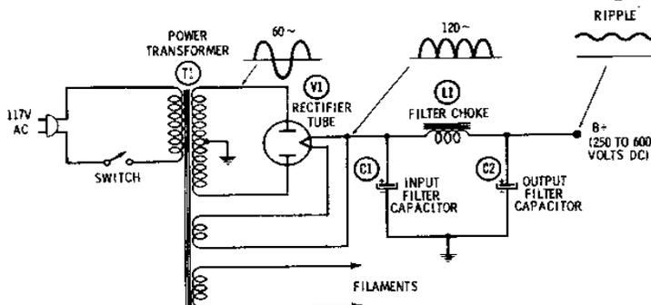
Fig. 5-3. Power-supply waveforms.
