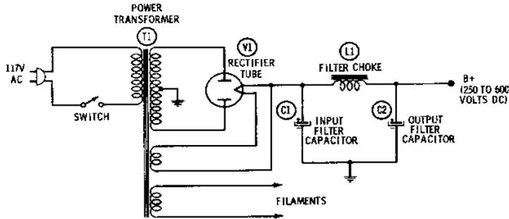
Fig. 5-2. Full-wave power supply using a power transformer.
