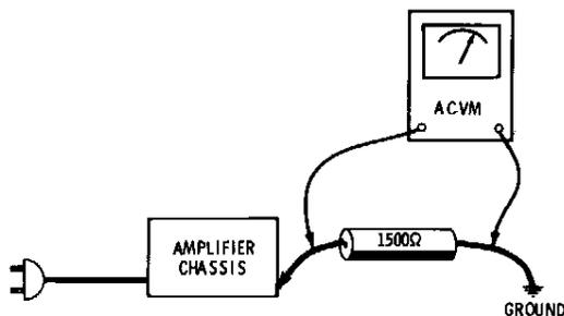
Fig. 3-10. Checking ac powered amplifier for a short to chassis.
