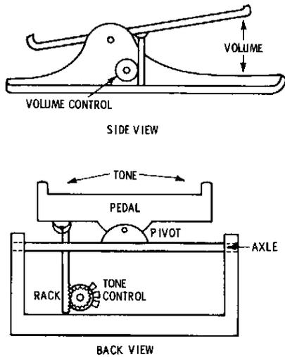
Fig. 8-9. Foot-operated tone and volume control mechanism.
