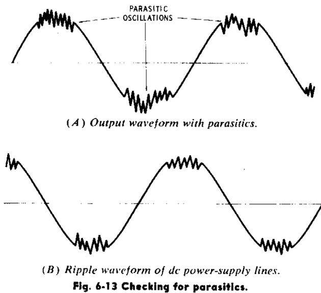
(A) Output waveform with parasitics.
