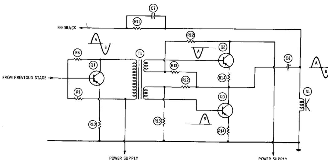
Fig. 1-9. Stacked output stage with an input transformer.
