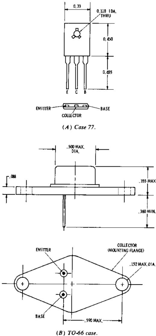
Fig. 4-8. Cases for low- and medium-power transistors.
