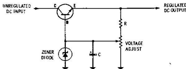
Fig. 5-9. Basic circuit of a transistor voltage regulator.
