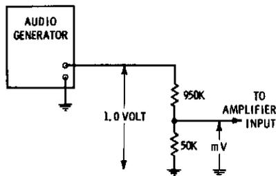
Fig. 8-4. Voltage divider to reduce generator output.
