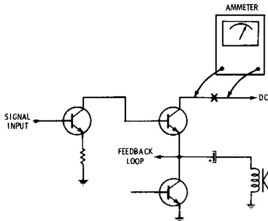
Fig. 6-7. Basic direct-coupled circuit.
