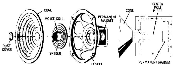
Fig. 6-16. Construction of a pm speaker.
